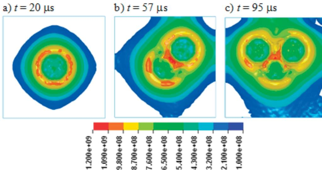
Fig. 7. Maps of the material effort [Pa] in a surface layer of the titanium alloy WT3-1 (Ti-6Al-2Cr-2Mo) after impact of: a) first ball, b) second ball, and c) third ball
