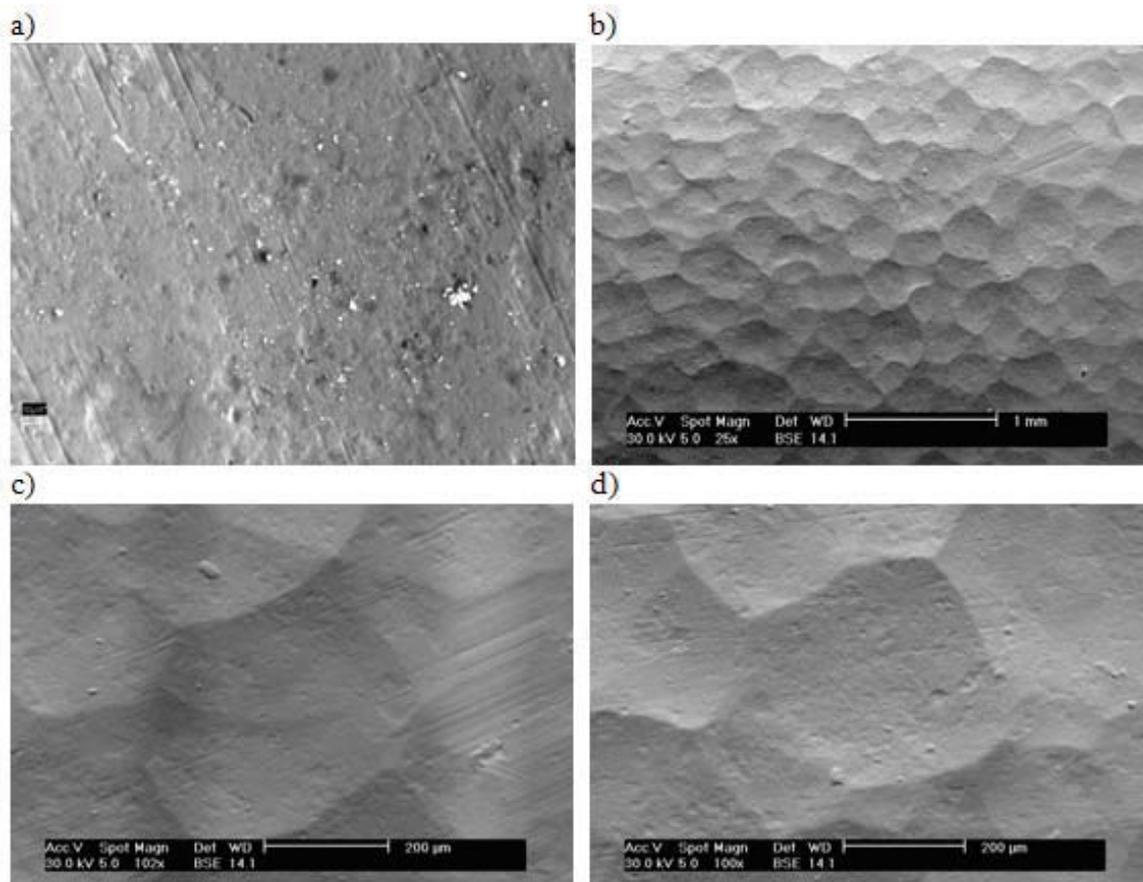
Fig. 3. A view of the characteristic surface topography zones of samples made of the titanium alloy WT3-1 (Ti-6Al-2Cr-2Mo) before and after shot peening: a) surface layer of the initial material before shot peening, b, c, d) surface layer of the material plastically deformed in result of the two-stage shot peening, scanning electron microscopy (SEM)
