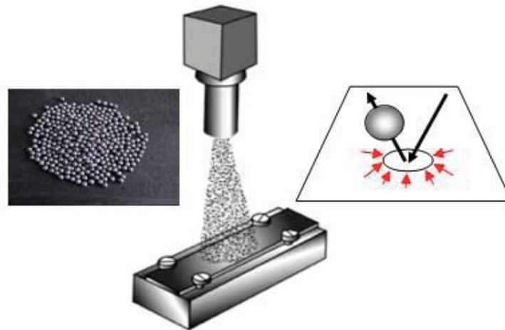
Fig. 1. Block diagram for mechanical shot peening using Almen testing plate
