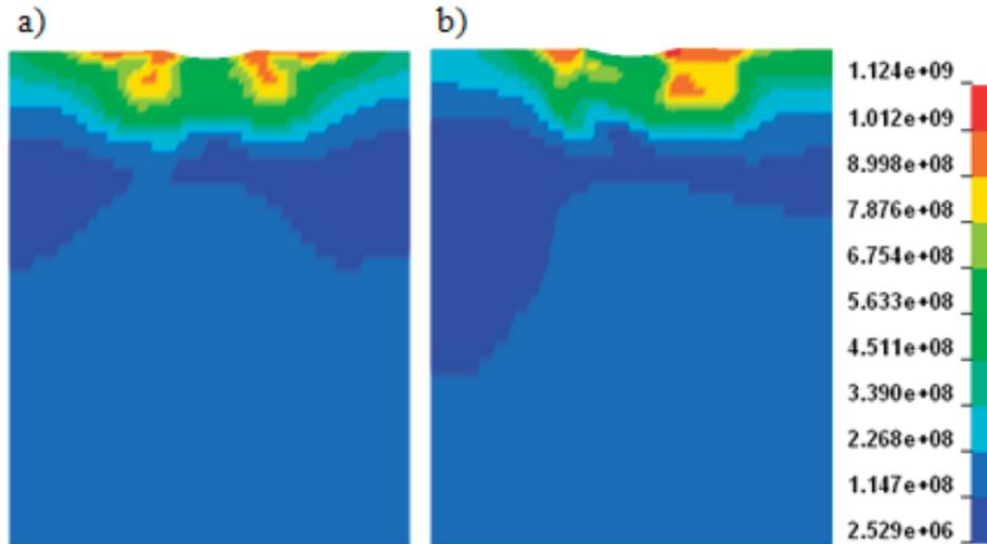
Fig. 6. Distributions of reduced stresses [Pa] for the C: a) – in the ZX plane, and b) in the ZY plane
