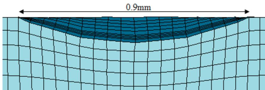
Fig. 5. A view of the plastically deformed zone generated in a process of mechanical interaction of a cast steel shot with surface layer of the titanium alloy WT3-1 (Ti-6Al-2Cr-2Mo)
