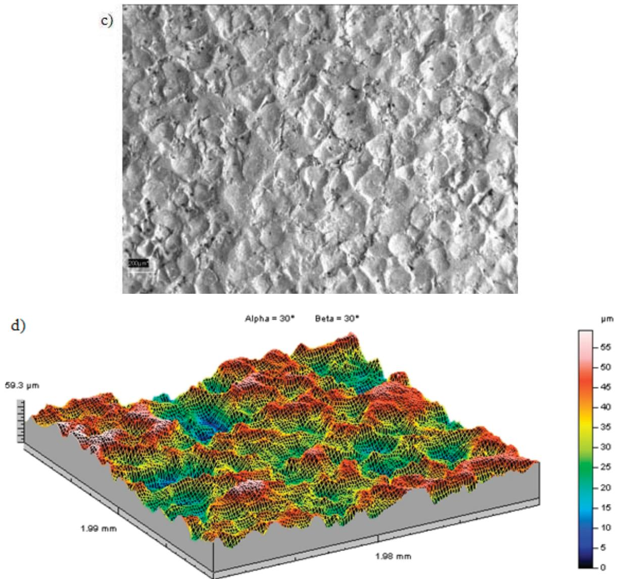
Fig. 2. Characteristic roughness profiles obtained from plane samples made of the titanium alloy WT3-1 (Ti-6Al-2Cr-2Mo): a, b) after mechanical shot peening – I stage (high intensity process –  $R_a \approx 75 \mu\text{m}$ ), c, d) – II stage (medium intensity process –  $R_a \approx 50 \mu\text{m}$ )
